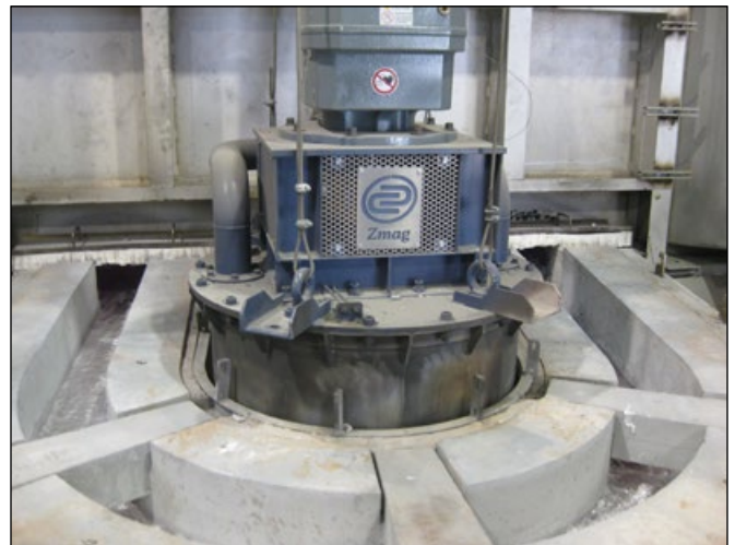
Figure 4. MagStir Series II stirrer with covers opened to show flow of metal through the canal.
